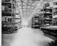
"Worm's eye" view of the warehouse, emphasizes the organized neatness of racked, palletized materials. The layout is designed with emphasis upon mechanical handling as with lift trucks and straddle trucks.
